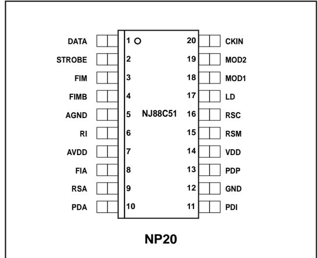
Fig.1 Pin assignment
